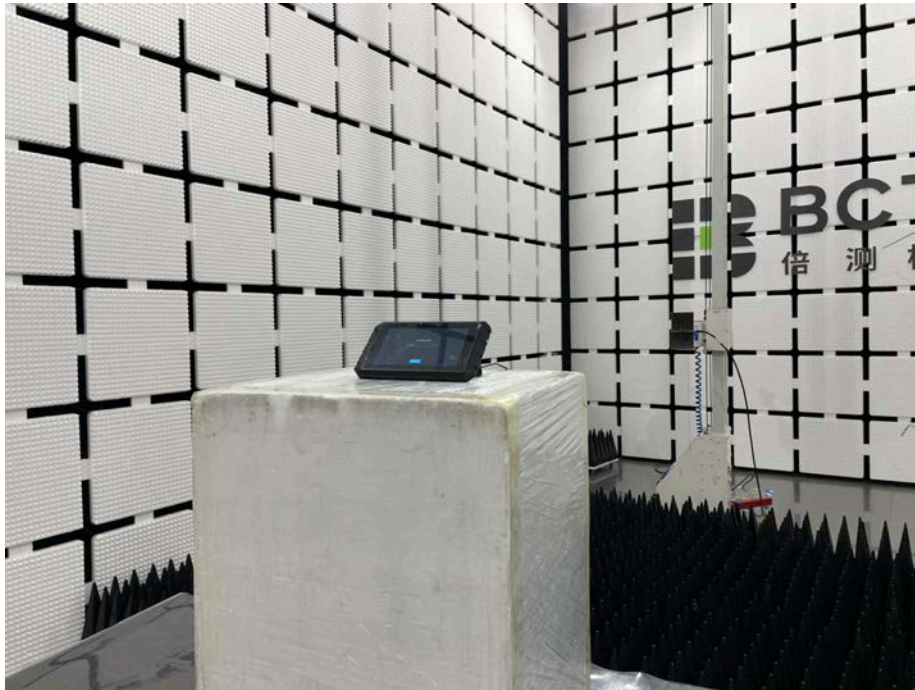
Spurious Emission Test Setup (above 1GHz)
