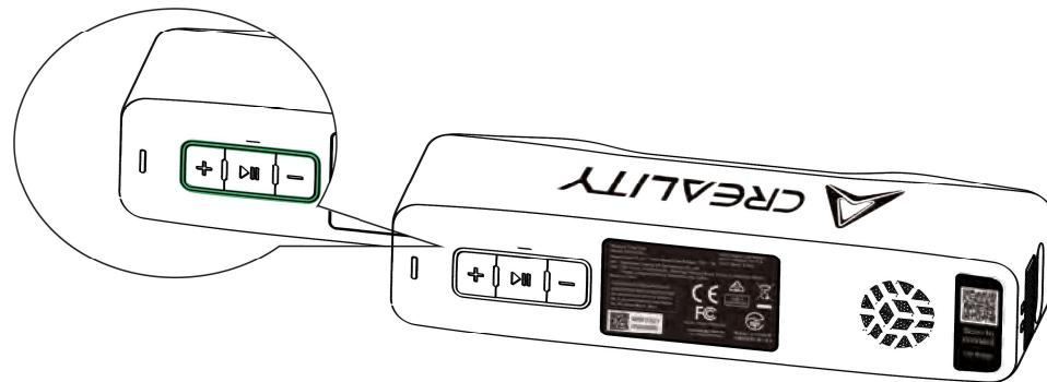
4. Short press ►|| on the scanner , or click "Start Scan" on the software interface to start scanning. Move the scanner slowly and try to keep the test piece in the center of the software preview window. Continue scanning until the model color turns green .
