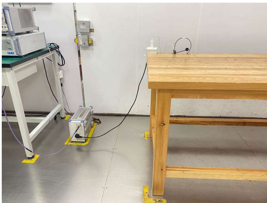
AC Power Line Conducted Emission Test Setup
