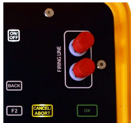
Figure 46. Firing line terminals
