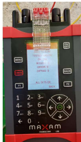
Figure 16. Connection between a RIOTRONIC+ detonator and RIOTRONIC X+ Logger
