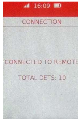
Figure 59. Blaster connected to Remote control device
