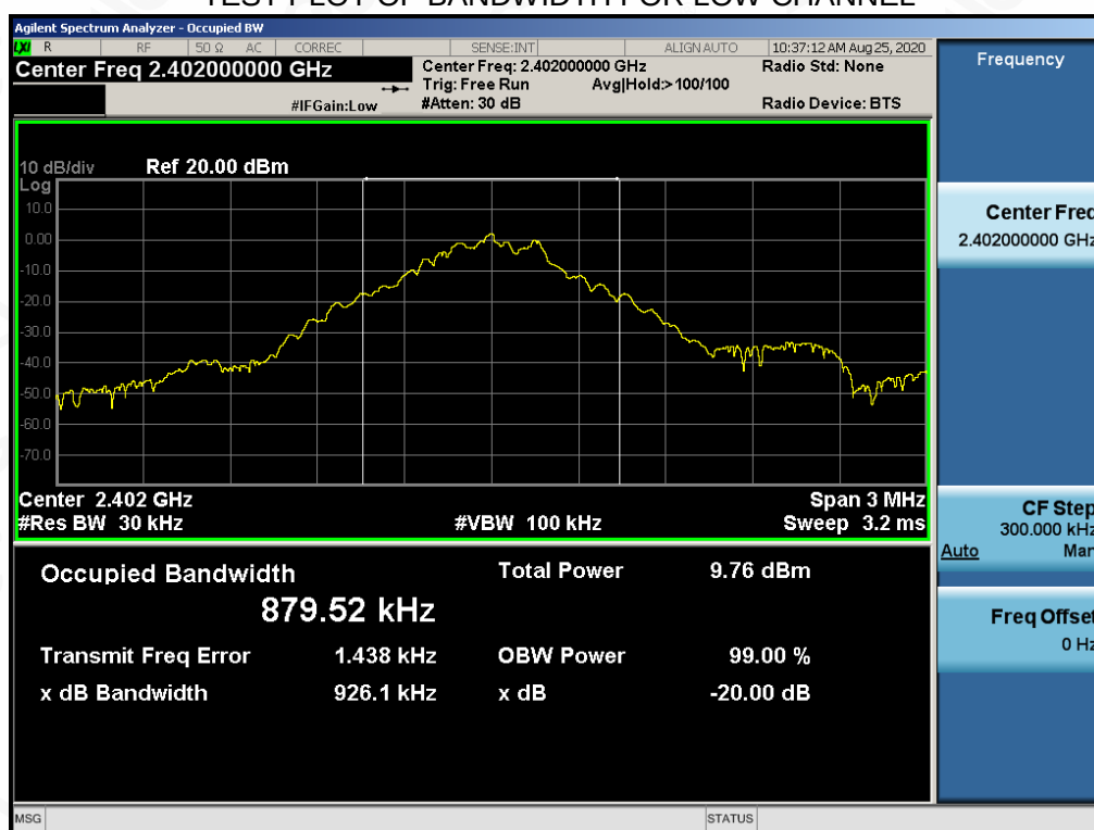
TEST PLOT OF BANDWIDTH FOR LOW CHANNEL
