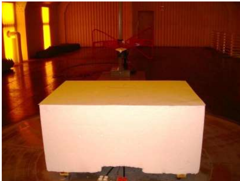
Photograph 10: Reference Photo of Test Setup for Emissions From 30 MHz to 1000 MHz
