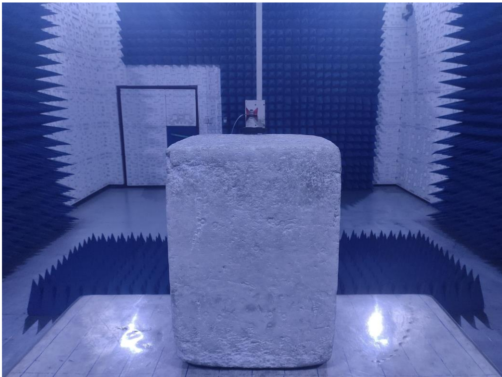
RADIATED EMISSION TEST SETUP ABOVE 1GHz
