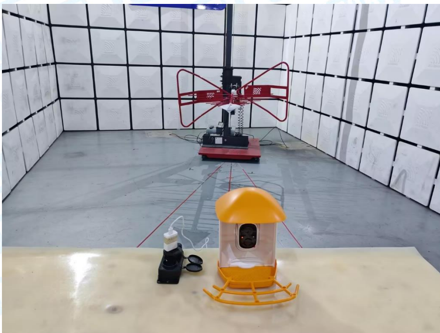
Photo of Setup for Radiated Emission (30MHz~1GHz)
