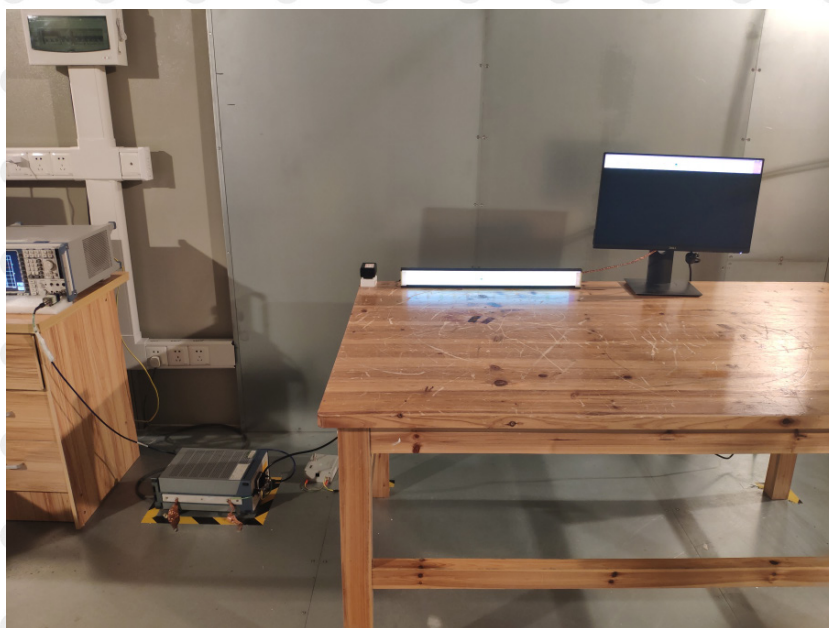
Photograph of test setup for Conducted Emission
