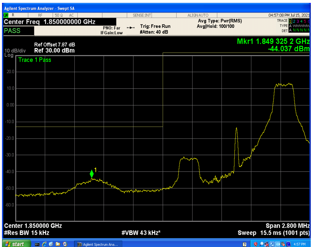
Band2 QPSK BW=1.4MHz Channel=19193 RB Size=1 Position=#0
