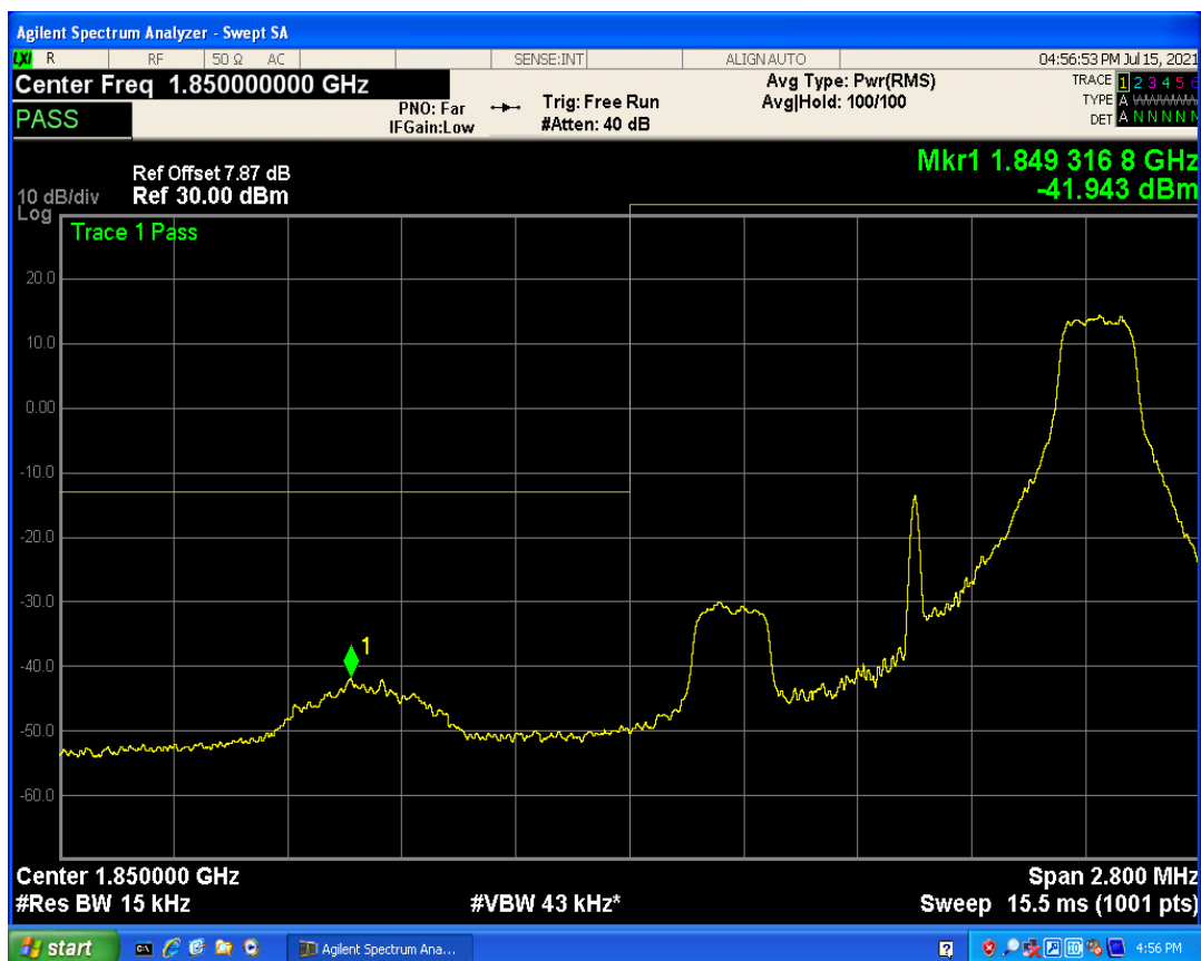
Band2 QAM16 BW=1.4MHz Channel=18607 RB Size=1 Position=#0
