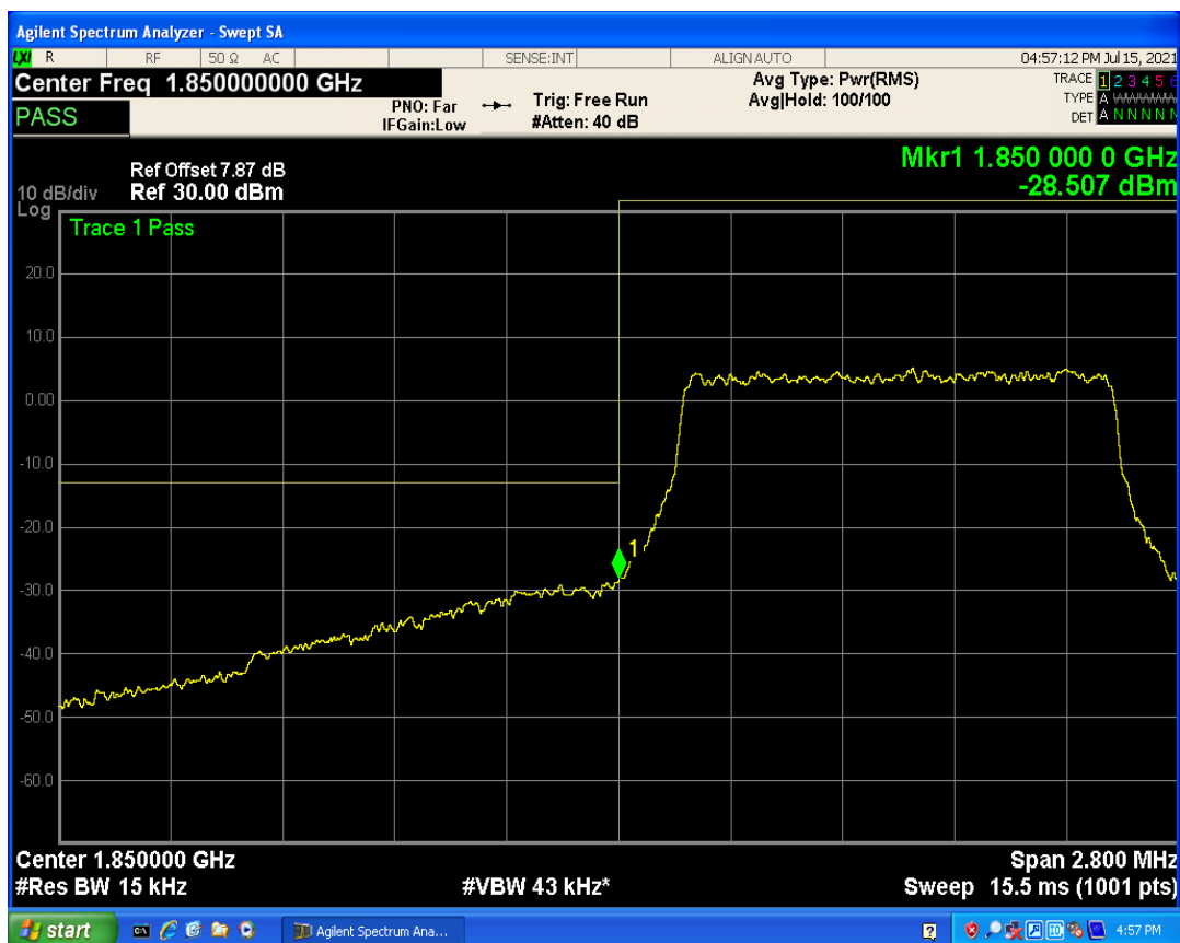
Band2 QPSK BW=1.4MHz Channel=19193 RB Size=1 Position=#Max
