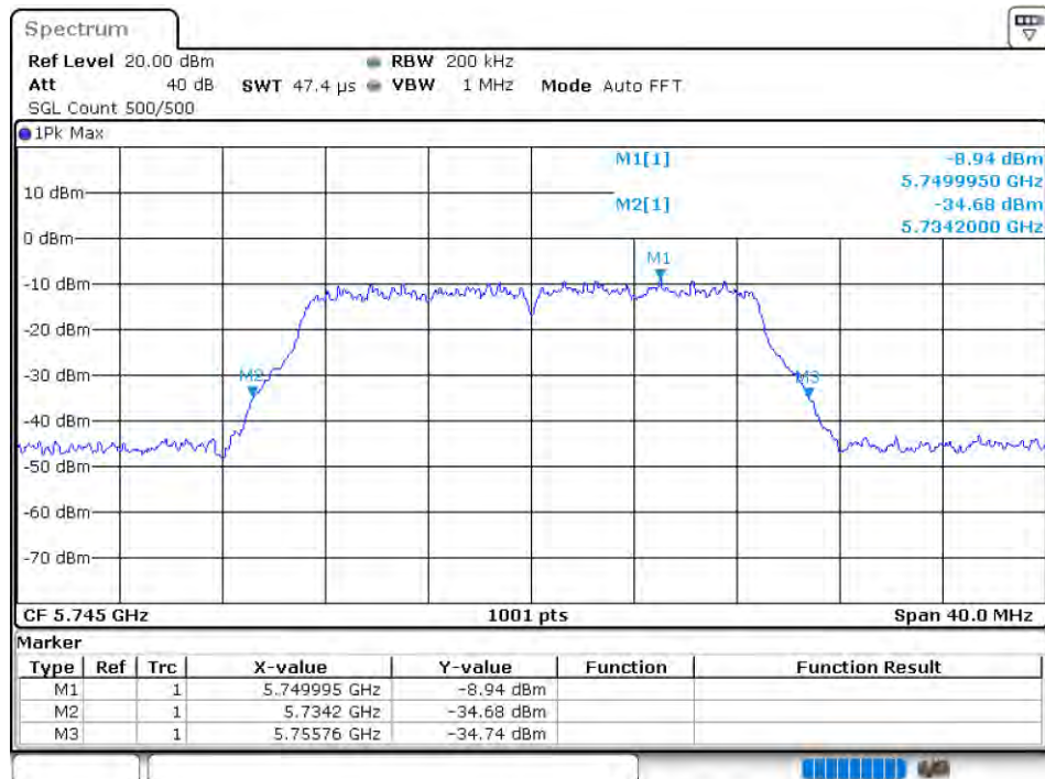
-26 dB BW NVNT 802.11n(HT20) 5745MHz Ant 2
