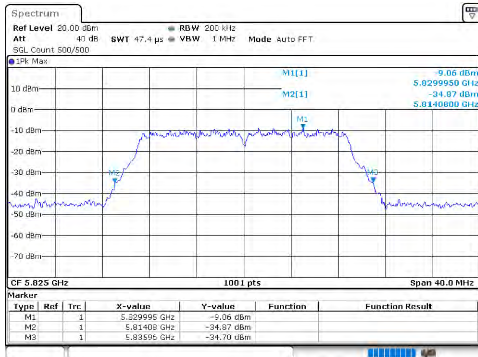
-26 dB BW NVNT 802.11n(HT20) 5825MHz Ant 1
