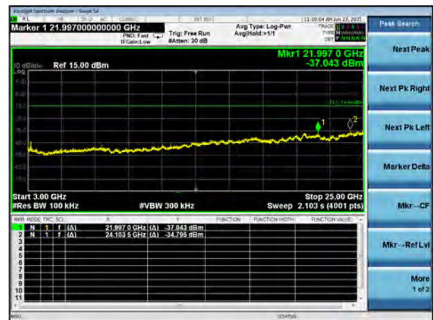
GFSK LOW CHANNEL, SPURIOUS 3 GHz ~ 25 GHz
