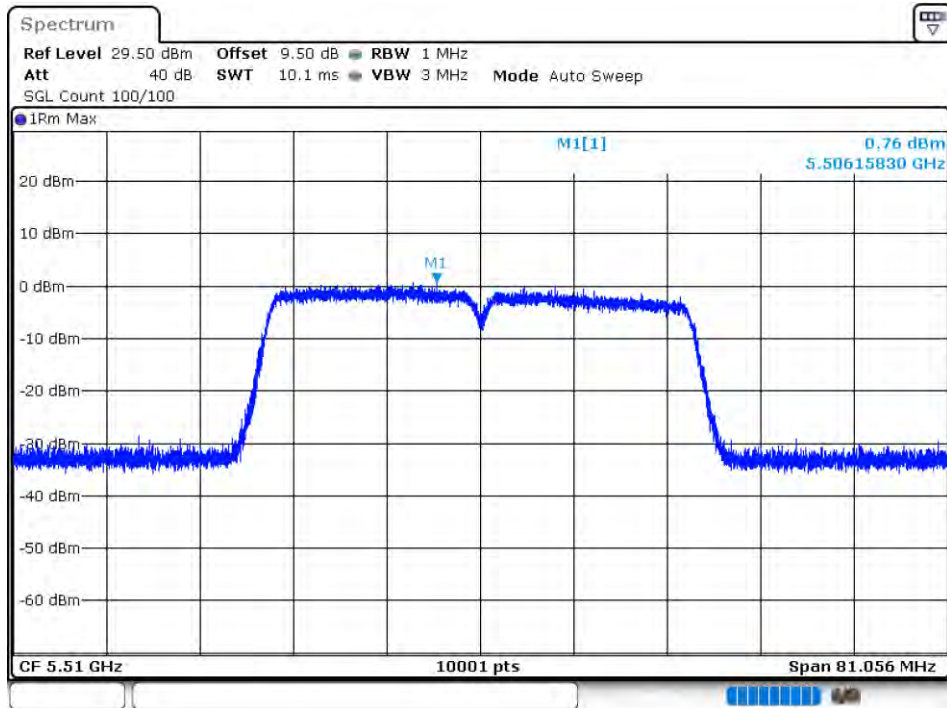
PSD NVNT 802.11ac40 5510MHz Ant 1
