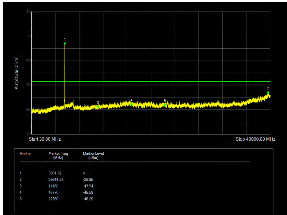
Tx. Spurious NVNT 802.11ac40 5590MHz Ant 1 Emission
