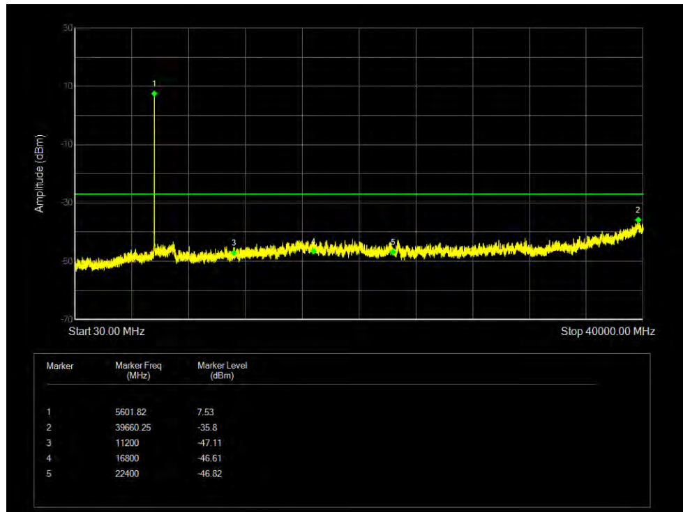
Tx. Spurious NVNT 802.11ac20 5600MHz Ant 1 Emission
