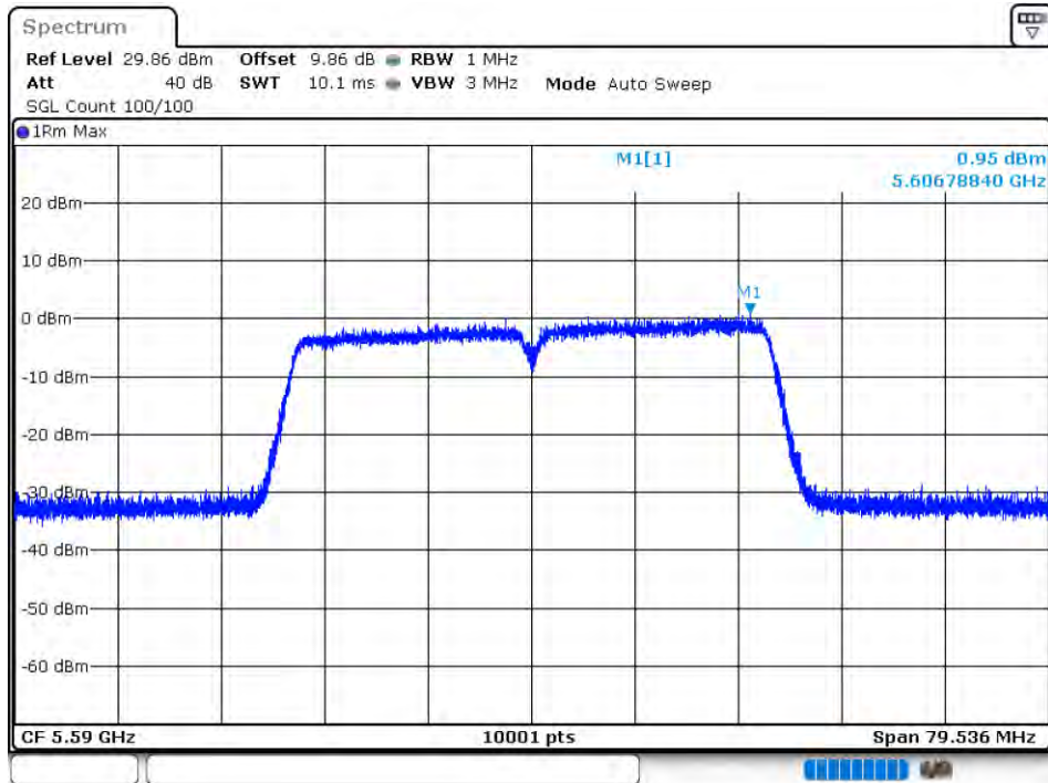
PSD NVNT 802.11n(HT40) 5590MHz Ant1
