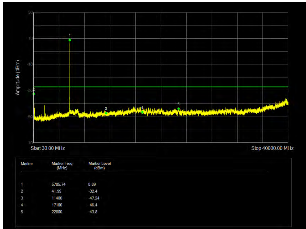
Tx. Spurious NVNT 802.11ac20 5700MHz Ant 2 Emission
