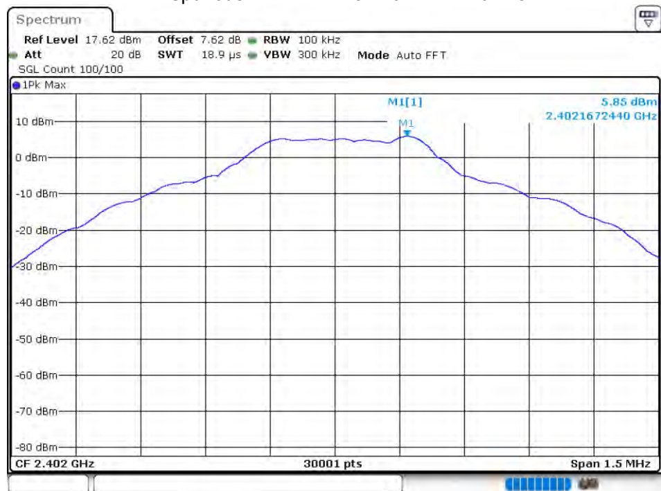
Tx. Spurious NVNT 1-DH5 2402MHz Ant1 Ref
