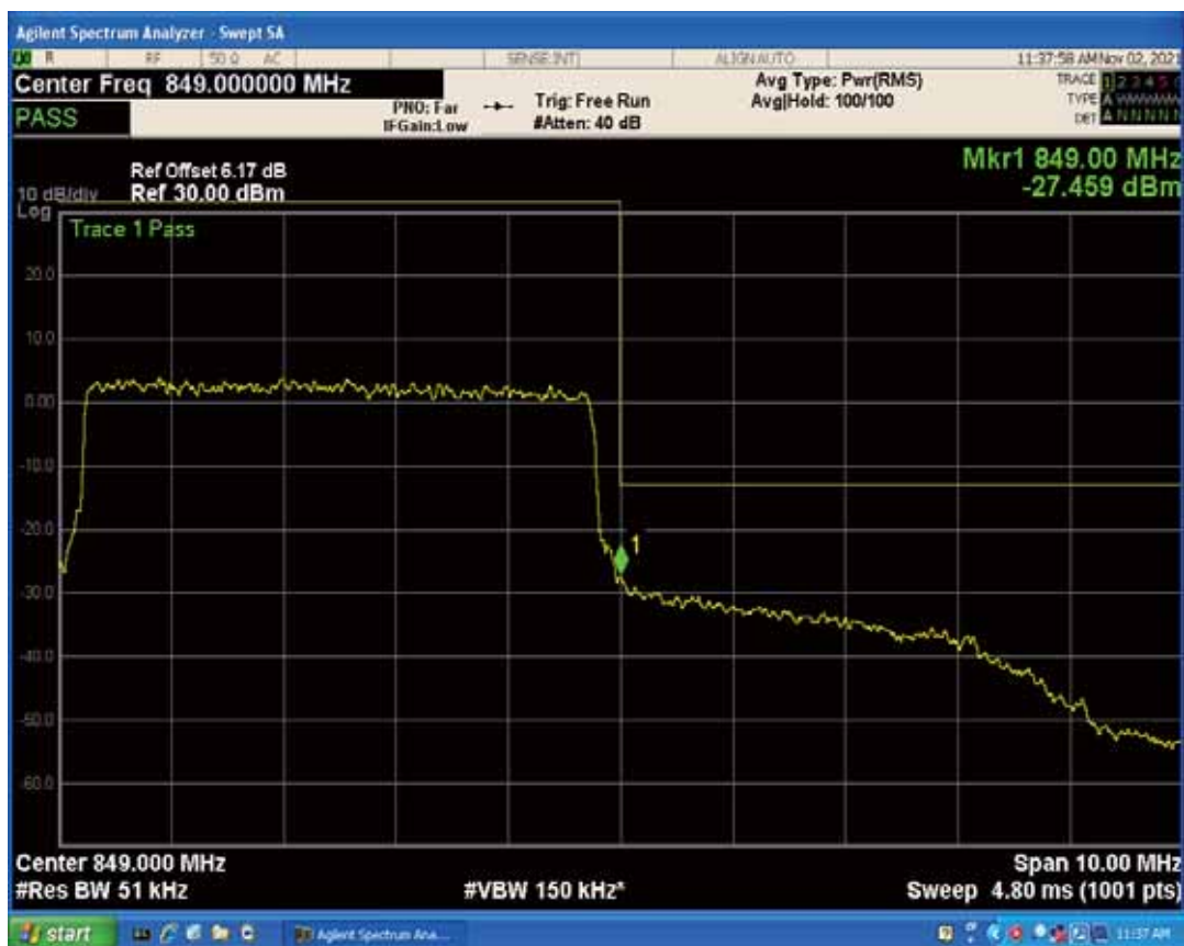
Band5 QPSK BW=10MHz Channel=20450 RB Size=1 Position=#Max
