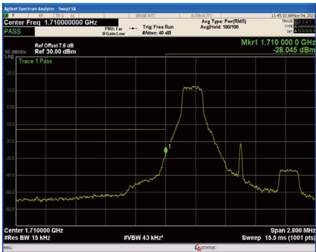
Band66 QPSK BW=1.4MHz Channel=131979 RB Size=6 Position=#0
