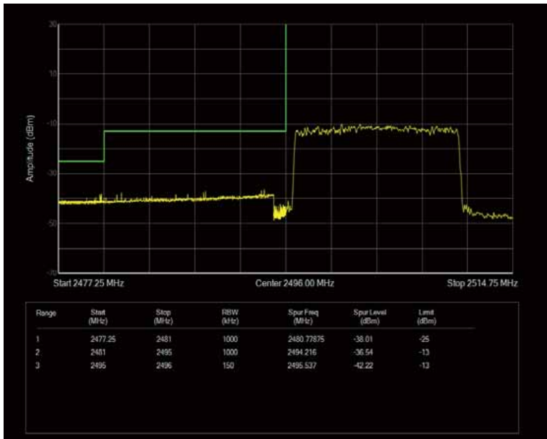
Band41 QPSK BW=15MHz Channel=41515 RB Size=1 Position=#Max
