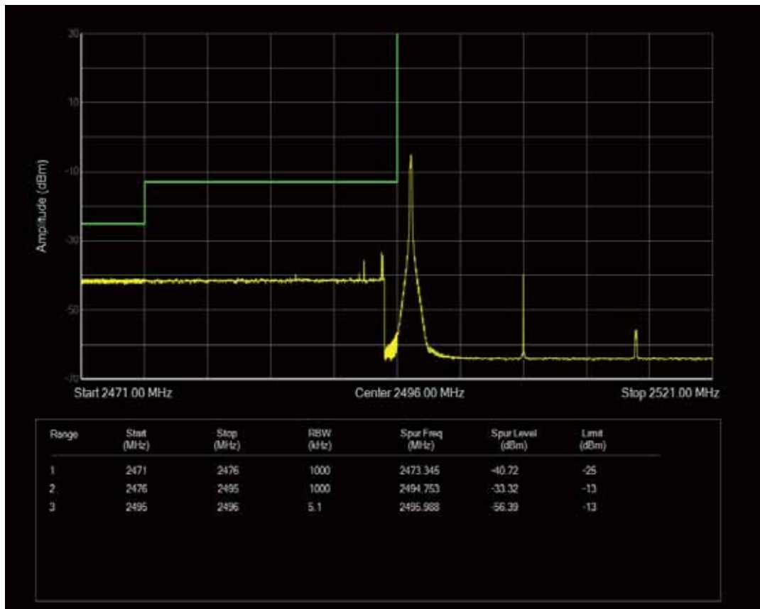
Band41 QPSK BW=20MHz Channel=39750 RB Size=100 Position=#0
