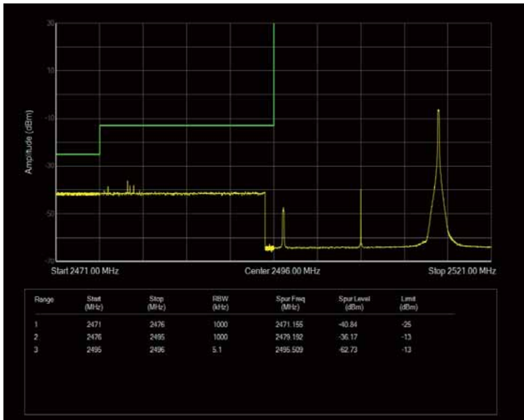
Band41 QAM16 BW=20MHz Channel=39750 RB Size=1 Position=#0
