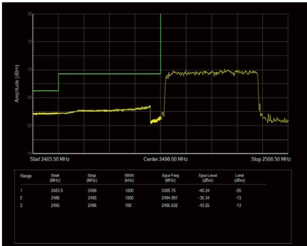
Band41 QPSK BW=10MHz Channel=39700 RB Size=50 Position=#0
