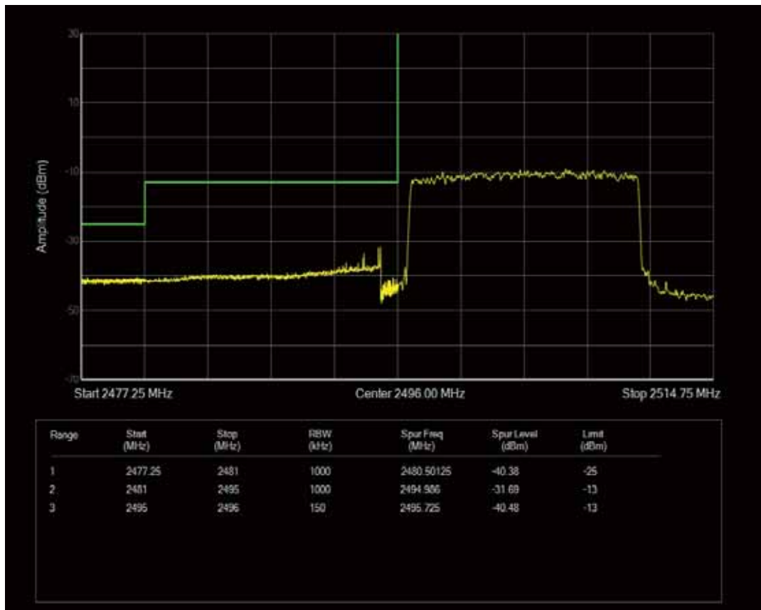
Band41 QAM16 BW=15MHz Channel=39725 RB Size=1 Position=#0
