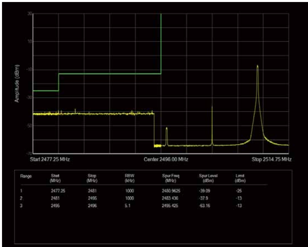
Band41 QPSK BW=15MHz Channel=41515 RB Size=1 Position=#0
