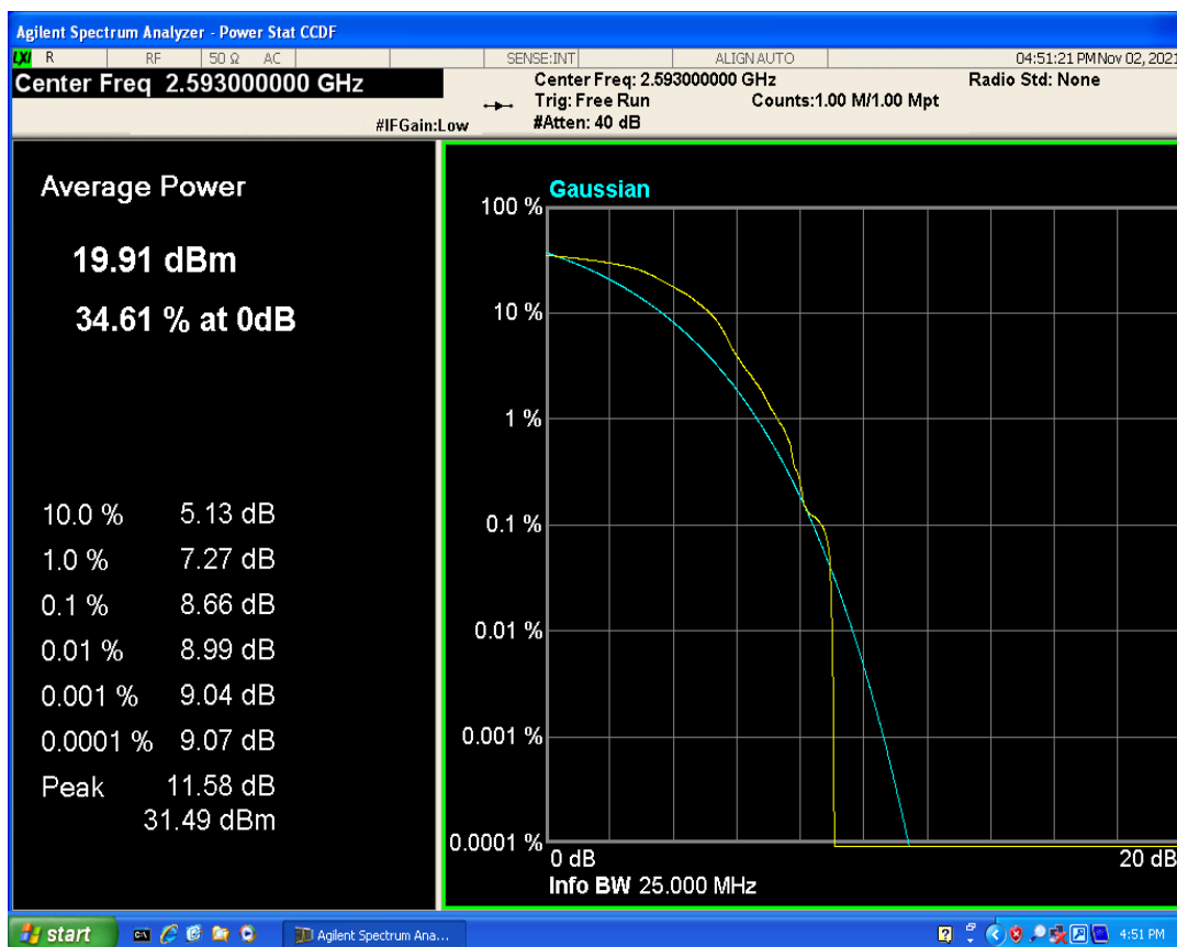
Band41 QPSK BW=15MHz Channel=40620 RB Size=1 Position=#0
