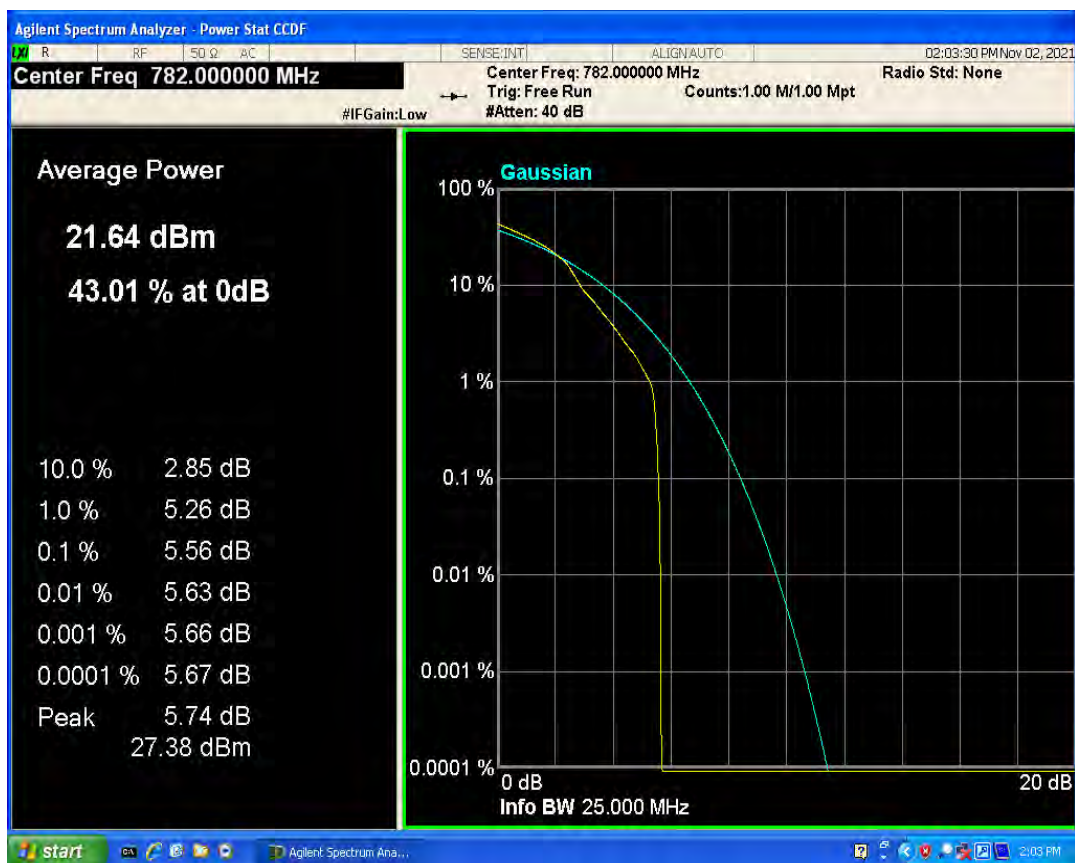
Band13 QAM16 BW=10MHz Channel=23230 RB Size=1 Position=#0
