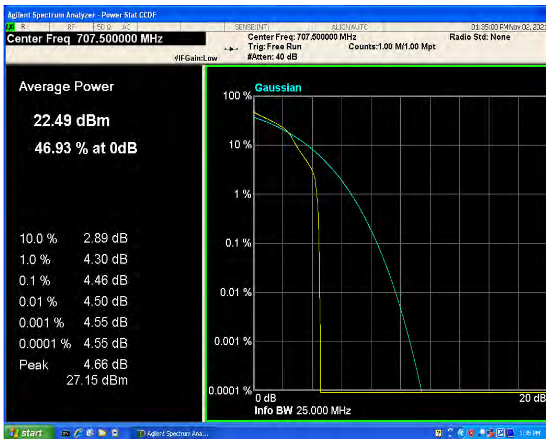
Band12 QAM16 BW=3MHz Channel=23095 RB Size=1 Position=#0
