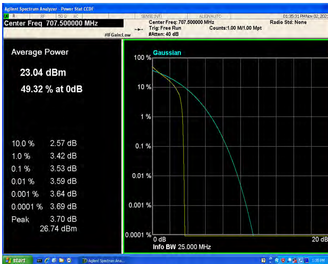
Band12 QAM16 BW=10MHz Channel=23095 RB Size=1 Position=#0
