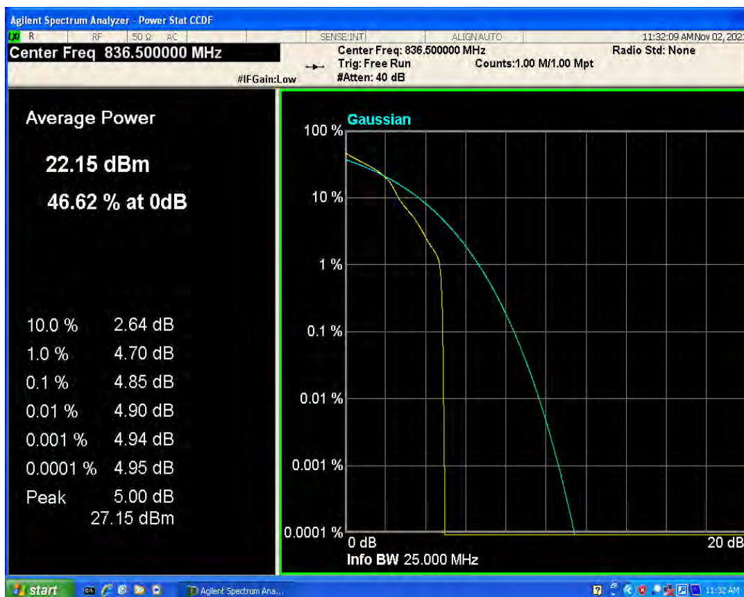
Band66 QPSK BW=1.4MHz Channel=132322 RB Size=1 Position=#0
