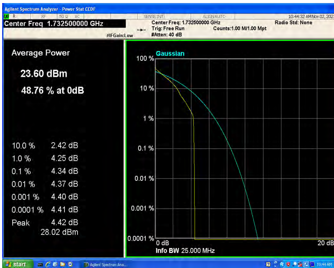
Band4 QAM16 BW=15MHz Channel=20175 RB Size=1 Position=#0
