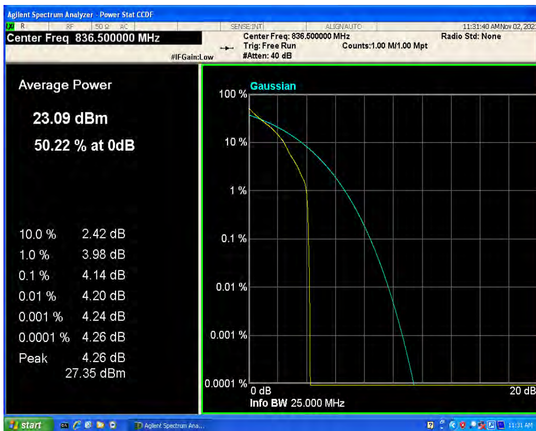
Band5 QAM16 BW=3MHz Channel=20525 RB Size=1 Position=#0
