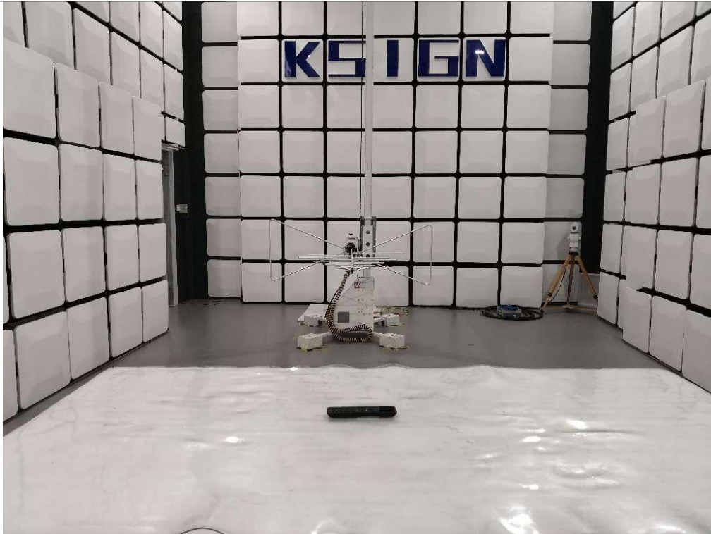
Radiated Measurement (Above 1GHz)
