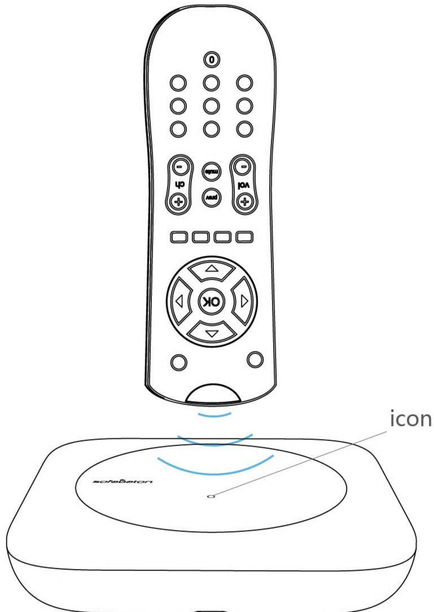
When learning, the original remote should be pointed toward the circular icon, at a distance of 3-5 inches and perpendicular to the hub surface.
