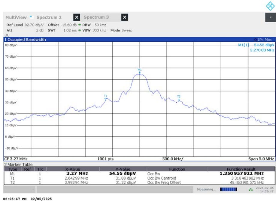
Plot 2: 6dB emission bandwidth MI e2eAudioHi mode
