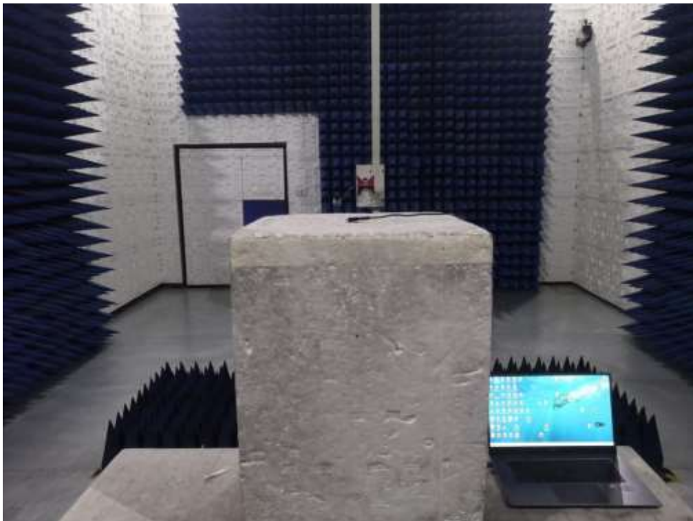
RADIATED EMISSION TEST SETUP ABOVE 1GHz
