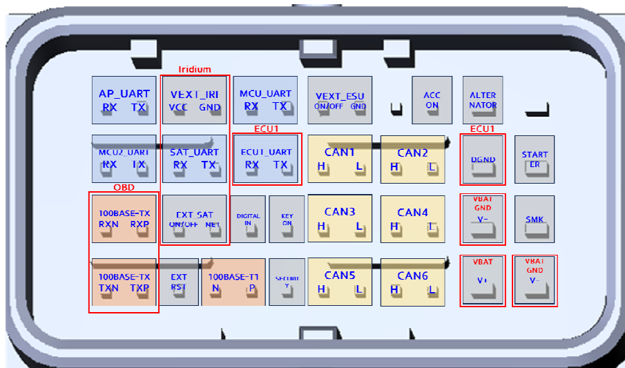
Fig. 3.7 Main Connector PINMAP1
