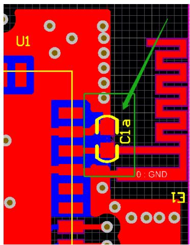
C1a is the antenna matching capacitance, which affects the signal strength. There is no need to paste here
