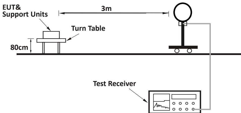
For Radiated emission 30MHz to 1GHz:
