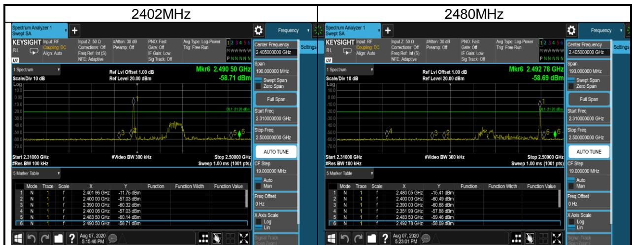
**TEST REPORT****7 Radiated Emissions in restricted frequency bands****Test result:** Pass**7.1 Limit**
