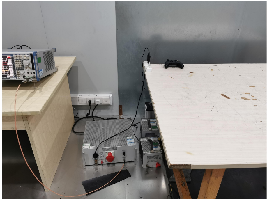
Conducted Emission Test Setup
