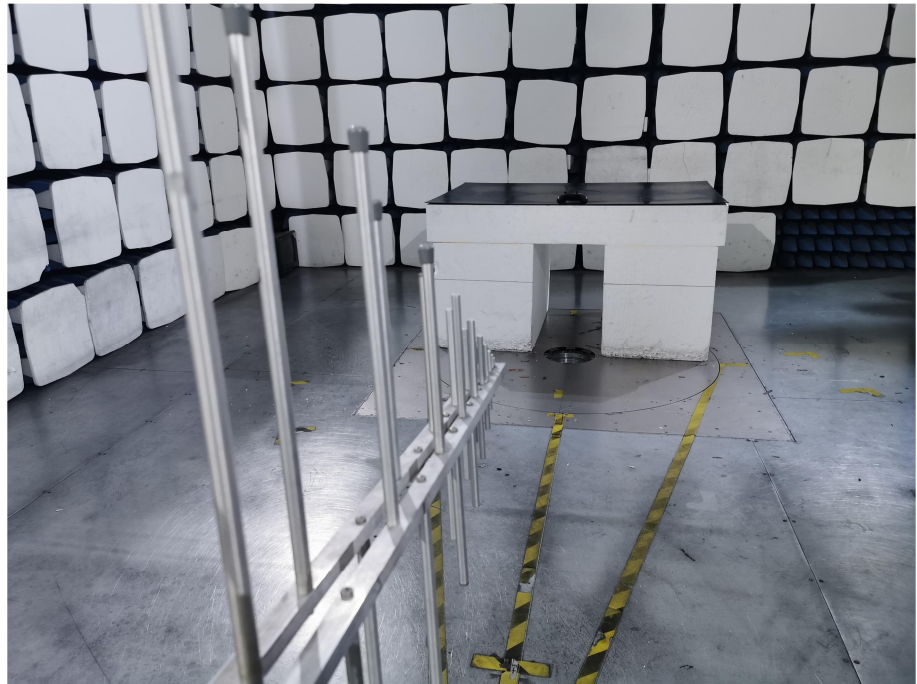
Radiation Emission Test Setup (30MHz to 1GHz)
