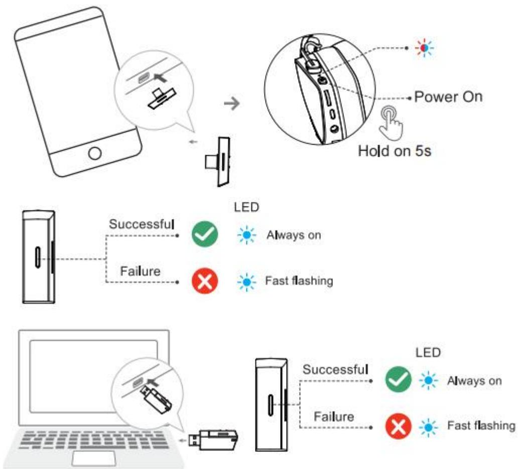
**Note:** Press and hold the power on button for more than 5 seconds , release your finger when you hear **Power On** and **Pairing**.
