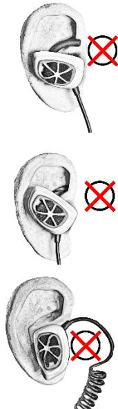
1. If the Ear Wing does not fully seat into the fold of the ear, the Ear Wing may be too large. Repeat “*WING AND FOAM FITTING*” steps 1-7 using the Small size Ear Wing.
