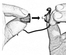
1. Orient the Foam Ear Tip so that the flat end is facing towards the Ear Piece and the rounded, tapered end is facing away from the Ear Piece.
