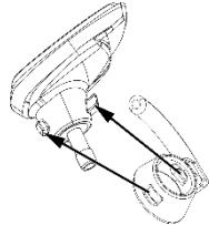
1. Orient the Ear Wing so that the rounded portion is facing towards the top and rear of the Ear Piece.
