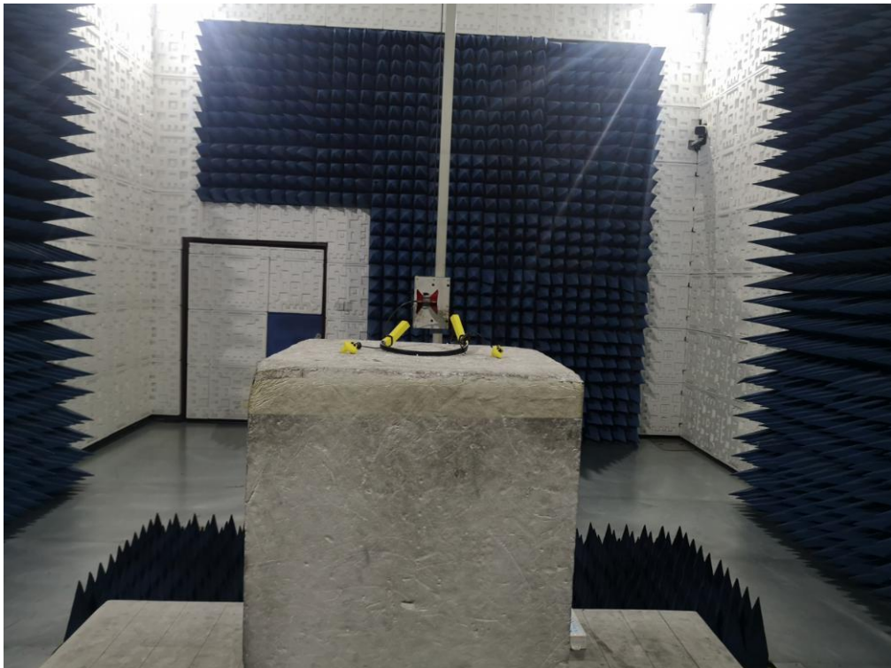
RADIATED EMISSION TEST SETUP ABOVE 1GHz
