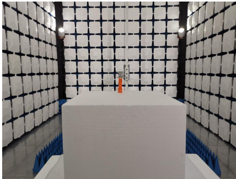
Above 1GHz for radiated emission test setup
