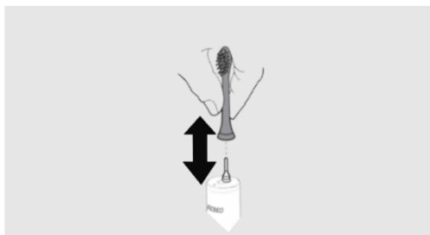
Reminder: (Do not press down the brush head hard when installing the brush head to avoid the malfunction of the extend-retract motor)
