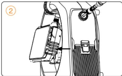
2. Extend the monitor stand by pulling it towards you for easier viewing access. **Or remove the monitor from the stand by unscrewing it from the back of the monitor.**
