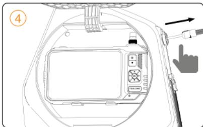
4. Pull out the inspection camera probe.
