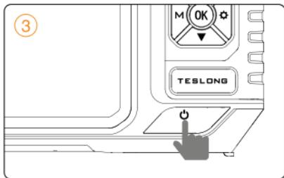
3. Press the power button to turn the monitor on. (Please make sure the TF card is installed before use.)
