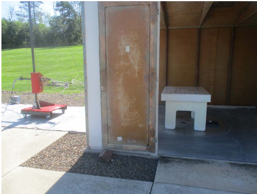
30 MHz to 200 MHz, Horizontal Polarization, Test Setup
