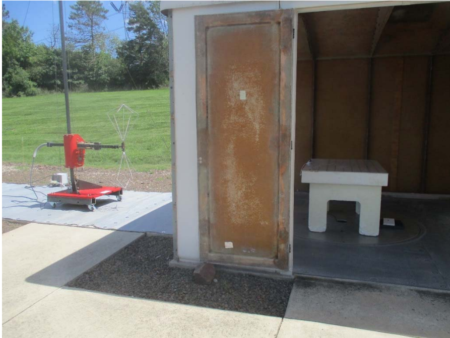
30 MHz to 200 MHz, Vertical Polarization, Test Setup
