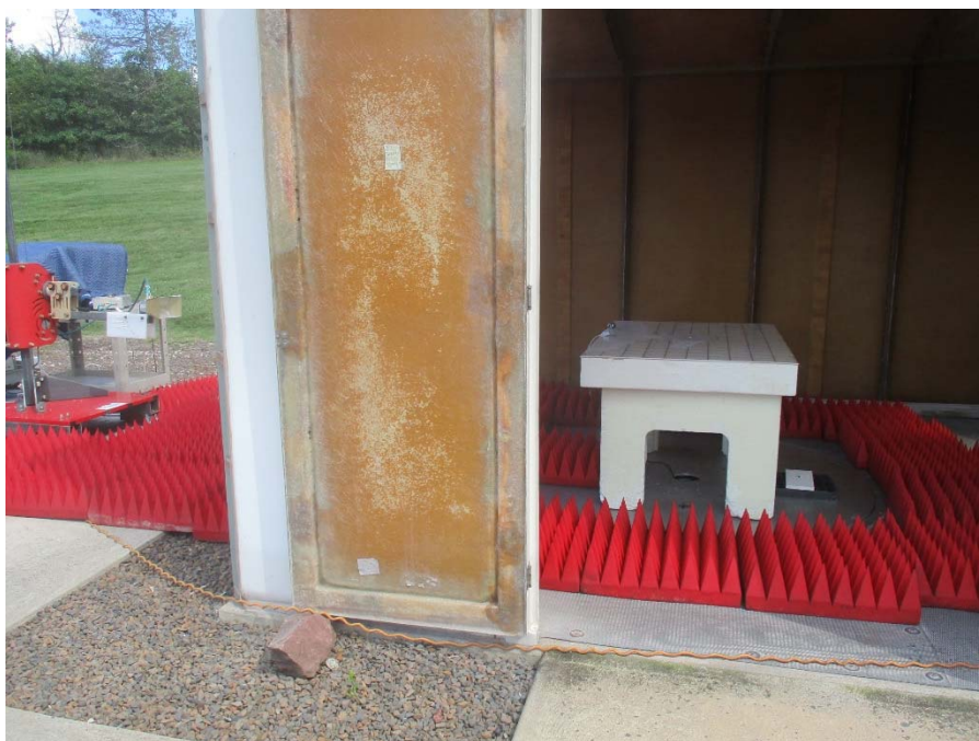
>1GHz, Vertical Polarization, Test Setup
