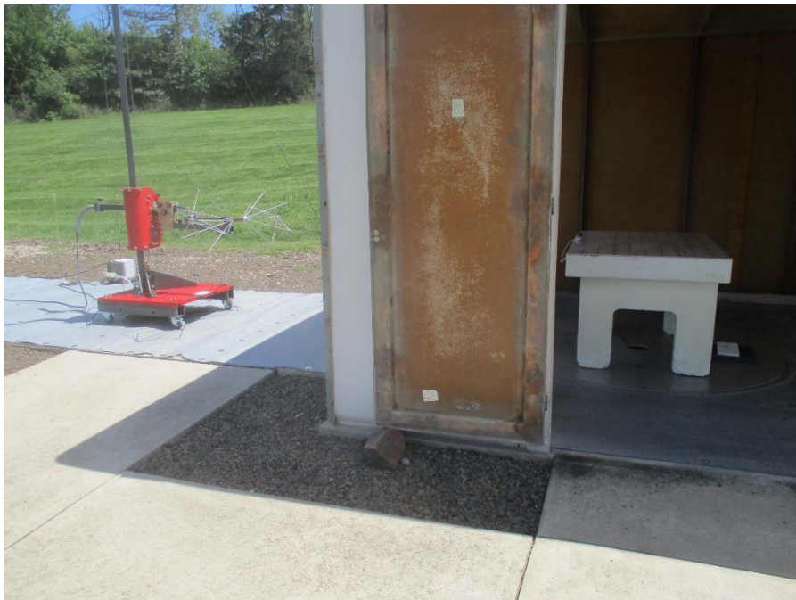
30 MHz to 200 MHz, Horizontal Polarization, Test Setup
