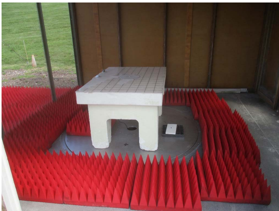
Above 1 GHz EUT Configuration
