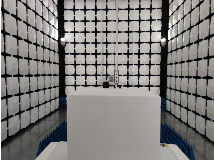
Below 1GHz for radiated emission test setup
