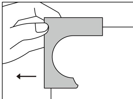
6. Remove the installation frame by sliding it to the left.
