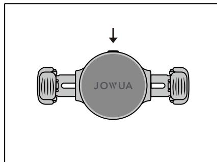
1. Press the button on the top of the car mount to release the side clamps.
