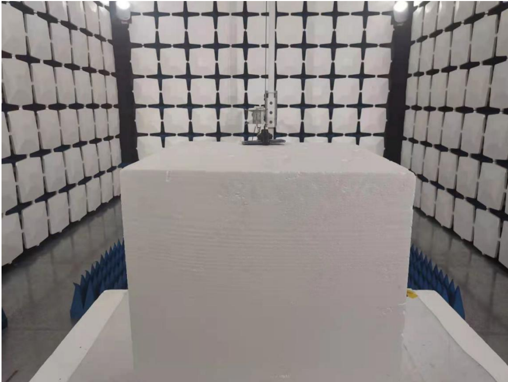
Above 1GHz for radiated emission test setup
