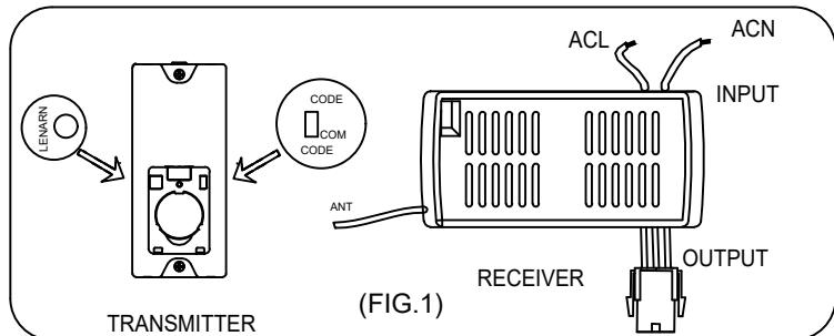
If there are two or more ceiling fans installed in the same house, in order to prevent your ceiling fans from being affected by the remote control of the adjacent ceiling fans, first turn the switch in each remote control transmitter to the CODE(UP) position (see the schematic diagram FIG1) Remarks: The standard state of the transmitter is in the down code COM.
