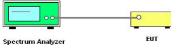
The EUT which is powered by the DC Power, is connected to the Spectrum Analyzer; the RF load attached to the EUT antenna terminal is 50 Ohm; the path loss as the factor is calibrated to correct the reading. Make the measurement with the spectrum analyzer's resolution bandwidth(RBW) = 100 kHz. In order to make an accurate measurement, set the span greater than RBW.
