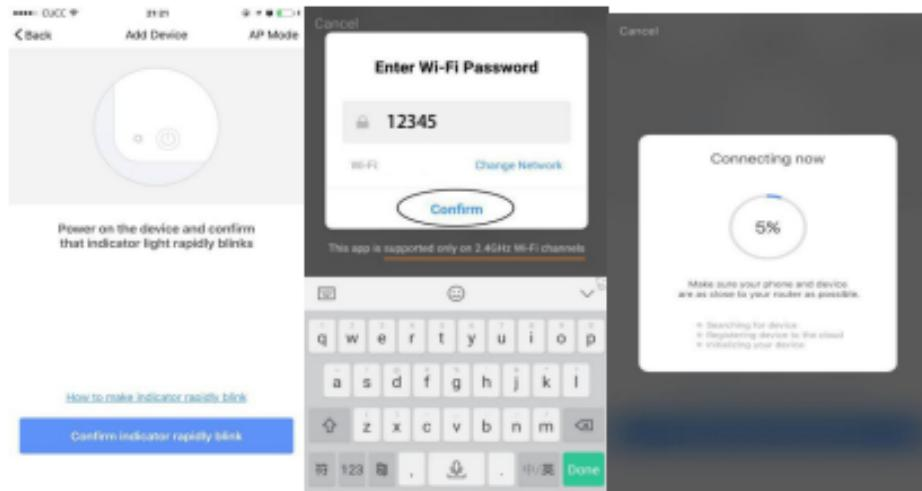
**Step 4:** Enter the device page, then complete the configuration.
