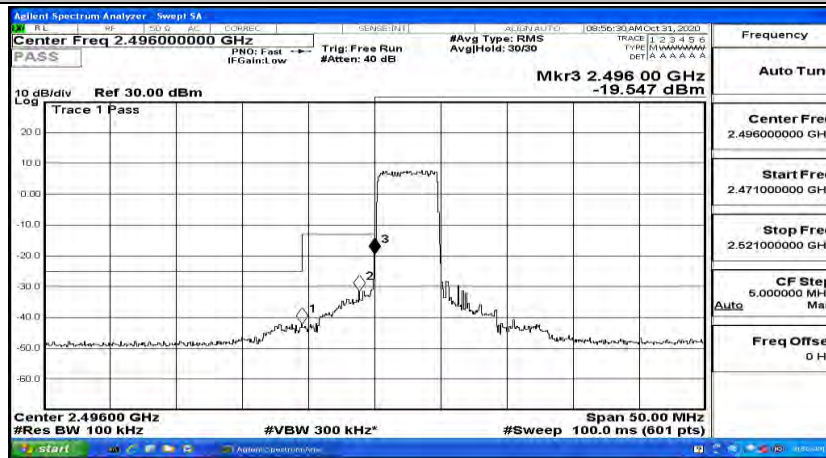
Band Edge Test Graph(s) (Channel Bandwidth: 5 MHz)_LCH_QPSK
