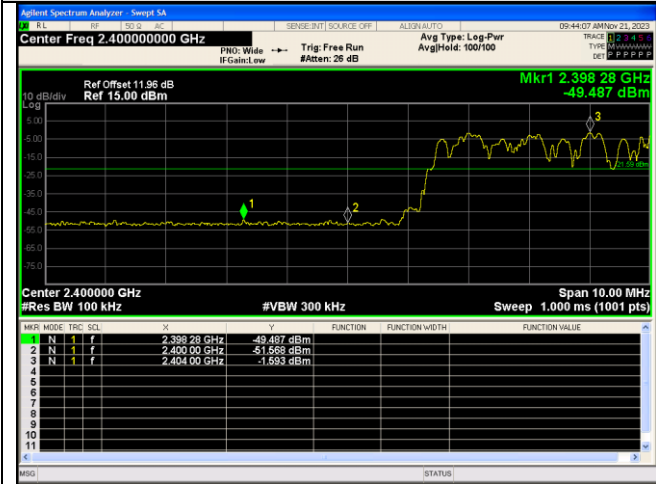
Out Of Band Emission(Left) 8DPSK_3-DH5_Channel Hopping
