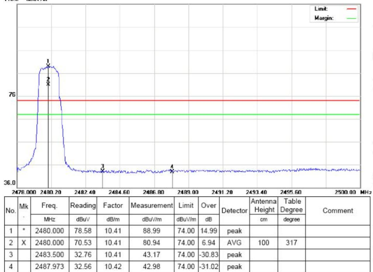
**Note:** Factor=Antenna Factor + Cable loss - Amplifier gain, Over=Measure-Limit.
