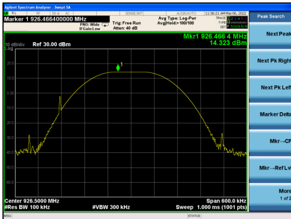
Peak output Power plot on channel 103 (1Mbps)
