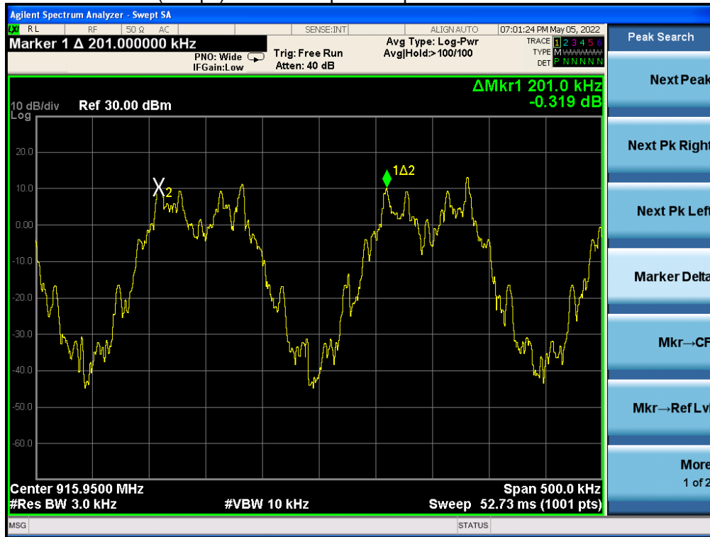
(1Mbps) Channel Separation plot on channel 102-103
