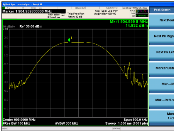
Peak output Power plot on channel 01 (1Mbps)
