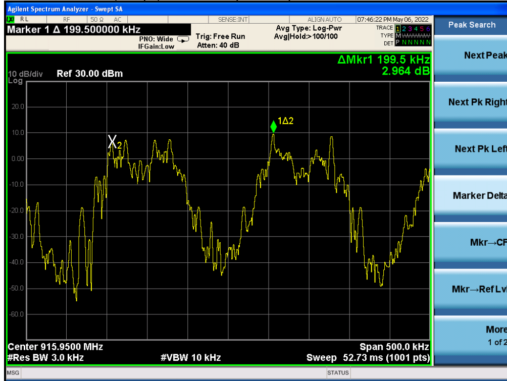
(1Mbps) Channel Separation plot on channel 102-103
