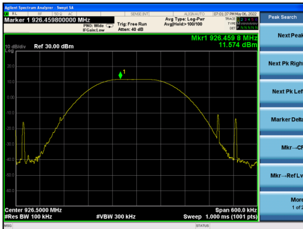
Peak output Power plot on channel 103 (1Mbps)
