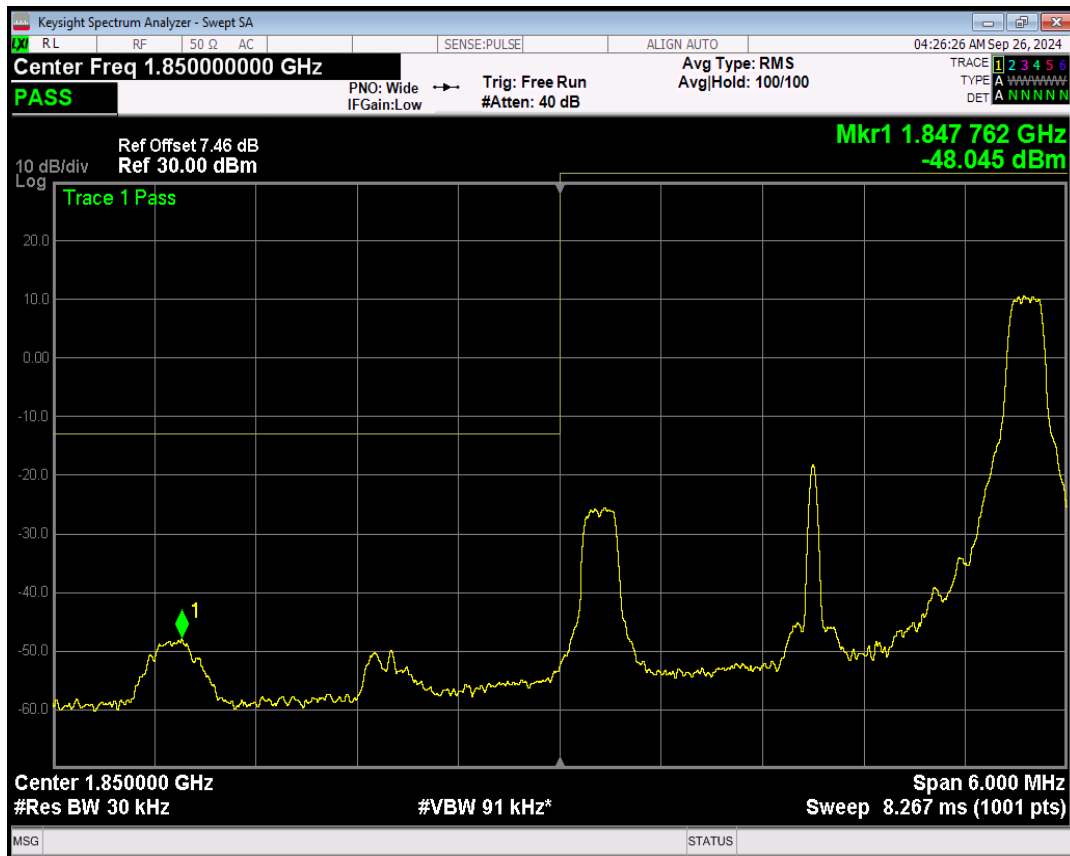
Band2 16QAM BW=3MHz Channel=18615 RB Size=1 Position=#0
