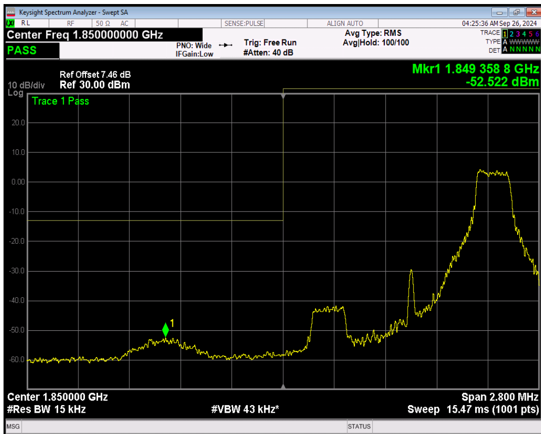
Band2 QPSK BW=1.4MHz Channel=19193 RB Size=1 Position=#0
