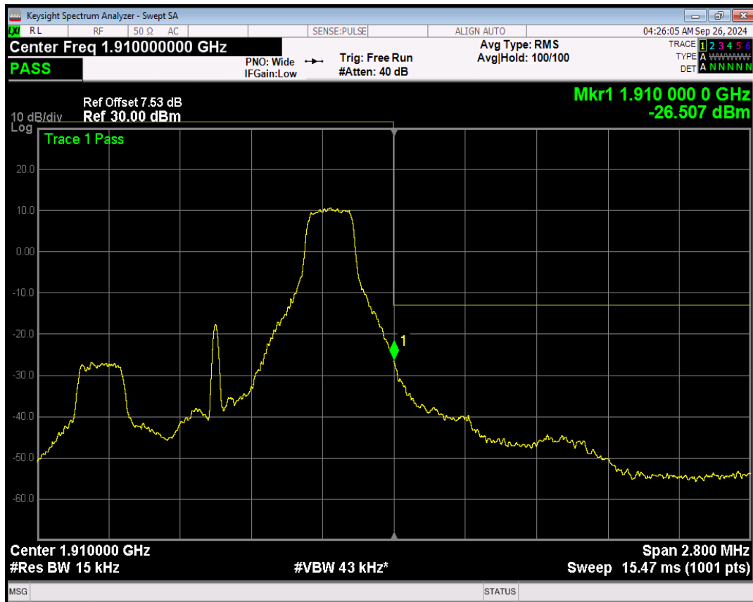
Band2 QPSK BW=1.4MHz Channel=19193 RB Size=6 Position=#0
