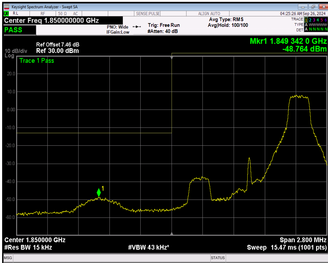
Band2 QPSK BW=1.4MHz Channel=18607 RB Size=6 Position=#0
