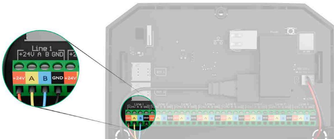
Hub Hybrid (2G) / (4G) has 8 Fibra lines. Numbers from 1 to 8 are indicated on the control panel board.
