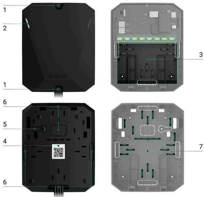
1. Screws that secure the casing lid. Unscrew with a bundled hexagon key ( $\varnothing 4$  mm).
