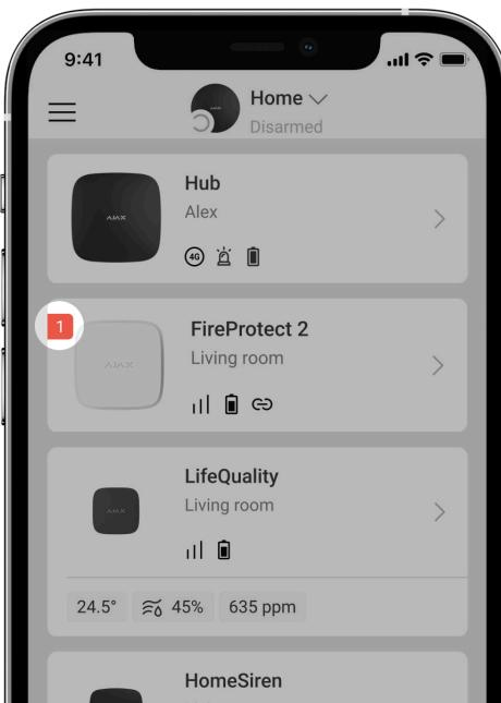
If FireProtect 2 malfunction is detected (for example, there is no connection with the hub), the malfunction counter is displayed in the device field in the Ajax apps.
