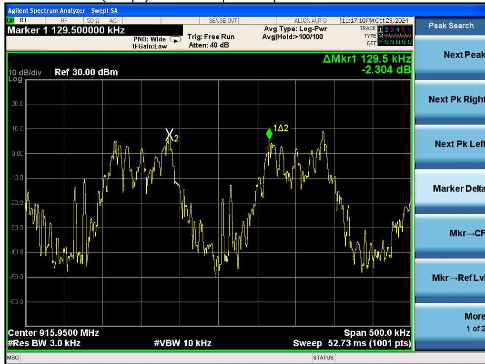
(1Mbps) Channel Separation plot on channel 102-103
