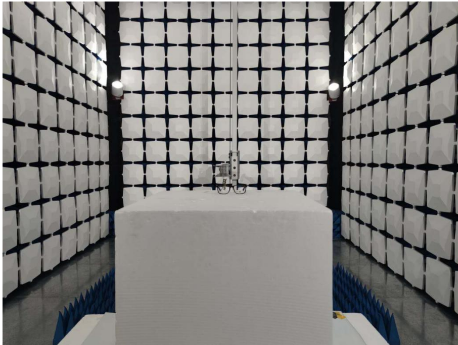
Below 1GHz for radiated emission test setup
