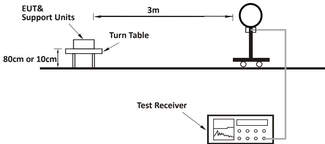
For Radiated emission 30MHz to 1GHz:
