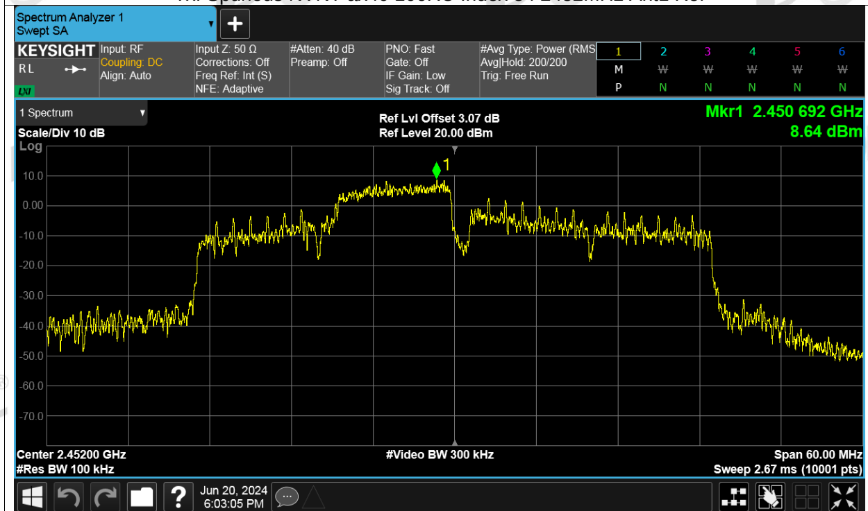
Tx. Spurious NVNT ax40 106RU Index 54 2452MHz Ant1 Emission
