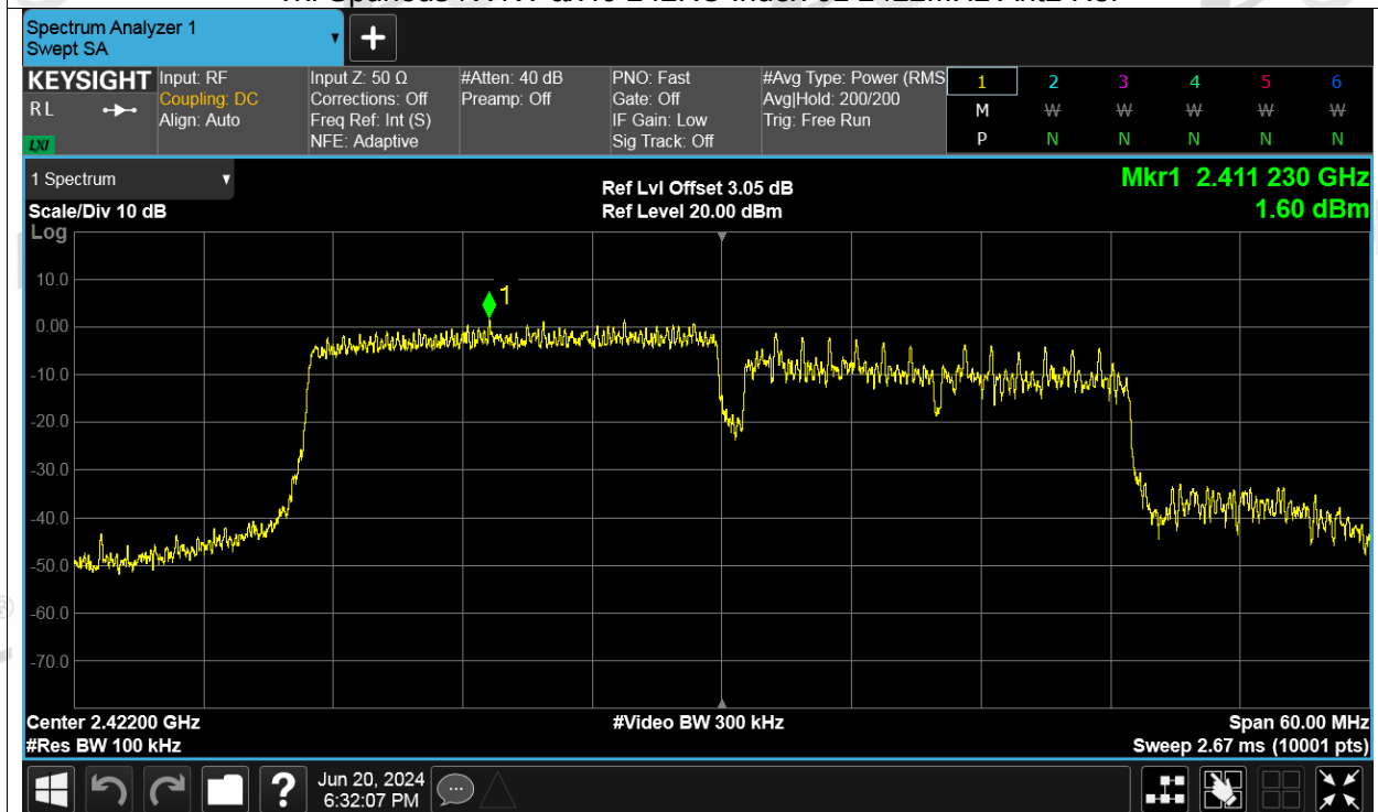
Tx. Spurious NVNT ax40 242RU Index 61 2422MHz Ant2 Emission
